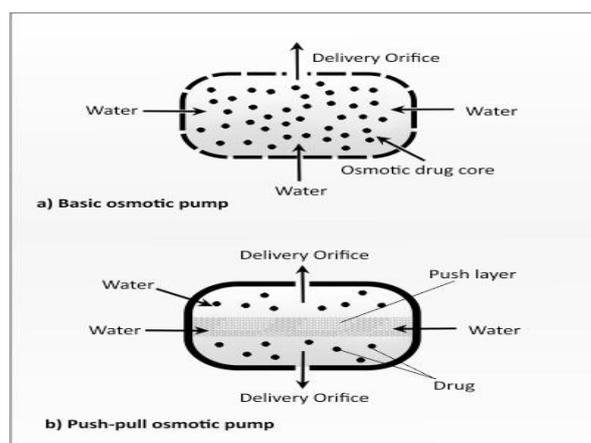
**Fig. 1.4:** Schematic representation of different types of osmotic pumps; (a) represents the basic osmotic pump and (b) represents the Push-pull osmotic pump.
