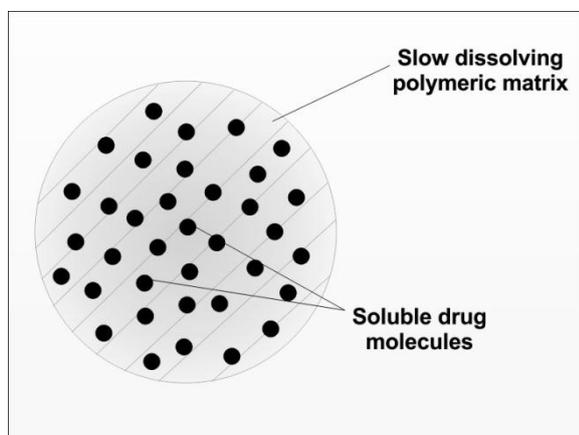
**Fig. 1.1:** Schematic diagram of the drug release from the reservoir system by dissolution of polymeric matrix.
