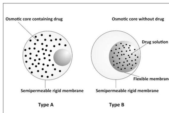
**Fig. 1.3:** Schematic representation of drug encapsulation in Osmotic system; Type A: Drug present in the osmotic core and Type B: Osmotic core without drug and the drug is present inside a flexible membrane.
