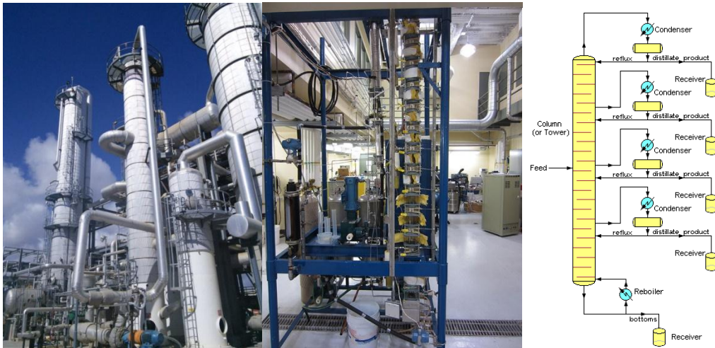
Figure 3: Continuous Distillation unit (Left: Industrial Basis, Middle: Laboratory Basis, Right: Diagram).
