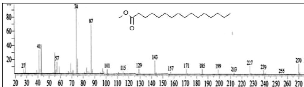
Fig. 3: Mass spectrum of hexadecanoic acid methyl ester.
