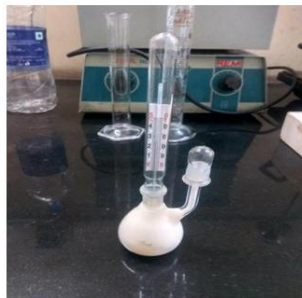
Fig 3: showing Pycnometer to calculate specific gravity
