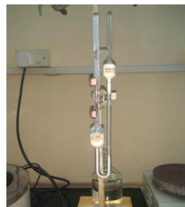
Fig 4:- showing Viscometer to calculate Viscosity.
