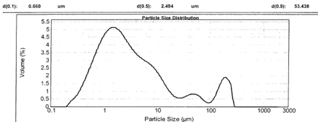
**Fig.7: Particle size distribution of Cefpodoxime Proxetil by Malvern technique.**
