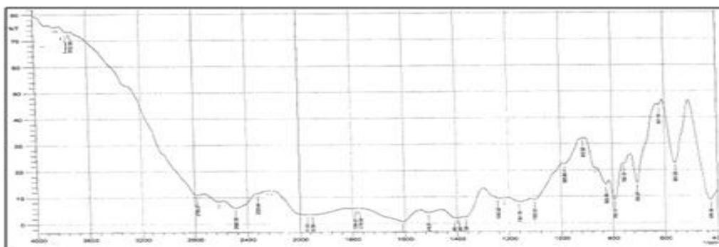
**Fig.8: FTIR spectrum of Cefpodoxime Proxetil with Xanthan gum**
