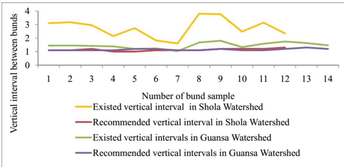
Figure 3: Existing vertical interval of bund against the recommended ones.
