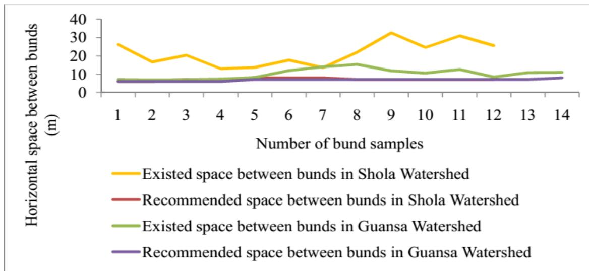
**Figure 2: Existing horizontal space of bund against the recommended ones**
