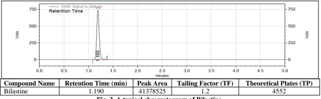
Fig. 3. A typical chromatogram of Bilastine.
