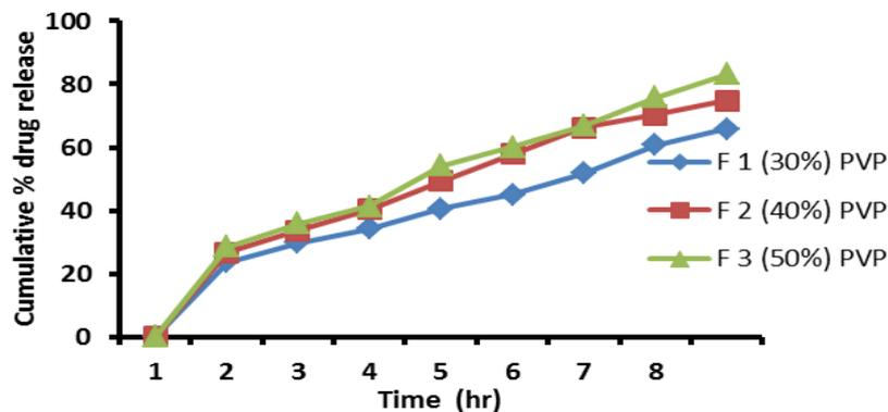
Figure 3: Comparison based on different pore forming %, *in vitro* cumulative drug release between F 1, F 2 and F 3\*.
