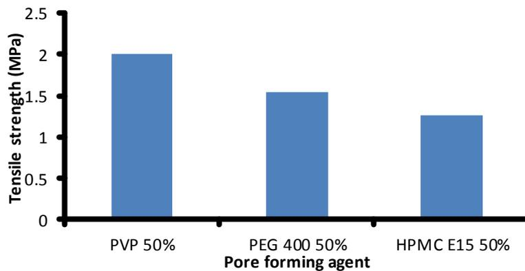
Figure 7: Strength of the membrane with different pore forming agents and thickness.
