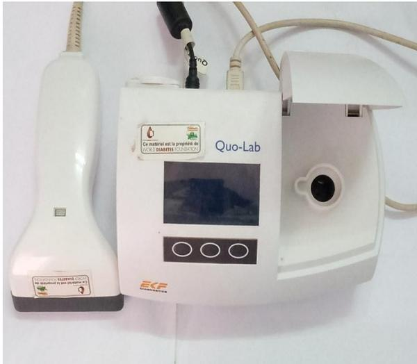
Figure 4: Apparatus for testing HbA1c glycated hemoglobin.
