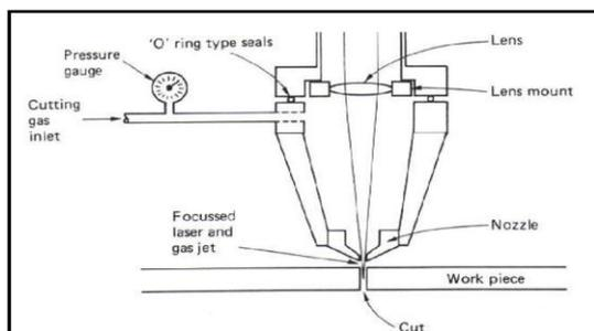
Figure: Laser cutting process.<sup>[16]</sup>
