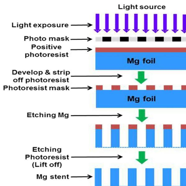
Figure: Manufacturing process of Photo Chemical Etching.
