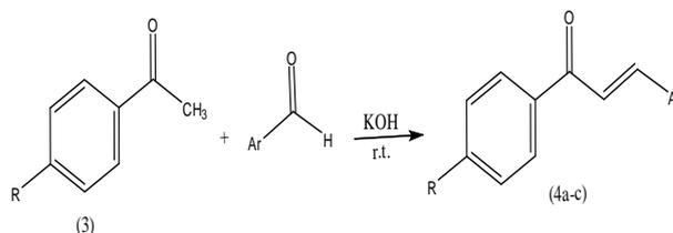
Figure 1: Synthesis of chalcone derivatives (4a-c).
