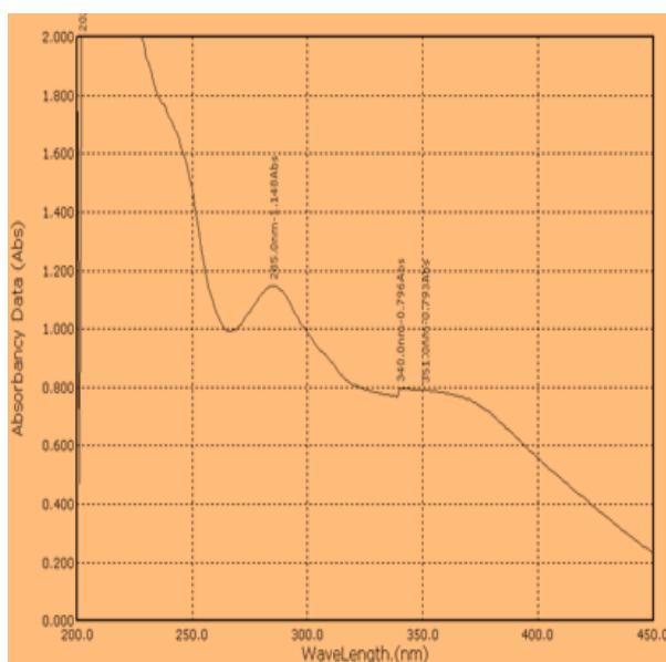
**Fig. 2: Sodium methoxide spectrum of compound I.**
