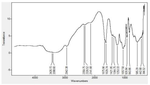
Figure 3: Spectrum of kappa carrageenan sample.
