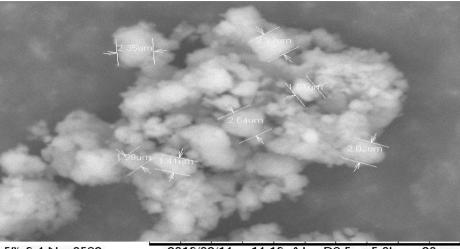
5% 6-4 Nes0582 2016/03/14 14:16 AL D8.5 ×5.0k 20 um Figure 4: Determination of particle size of the chondroitin sulfate powder.
