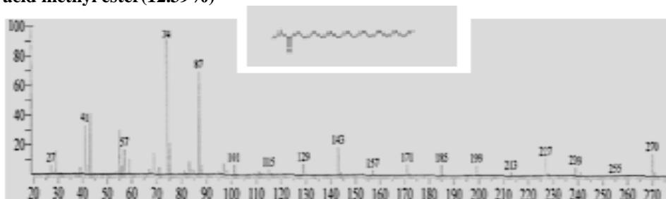
**Fig. 4: Mass spectrum of hexadecanoic acid methyl ester.**
