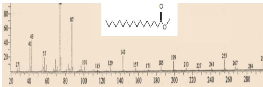
Fig. 6: Mass spectrum of methyl stearate.
