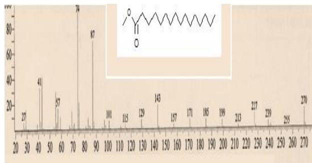
**Fig. 5: Mass spectrum of hexadecanoic acid methyl ester.**
