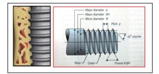
Thread pitch is the distance between two adjacent thread crests. Decreased thread pitch increases the functional surface area. More the number of threads, more is the surface area.
