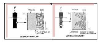
Threads on the implants improve initial stability, enlarge implant surface area and distribute stress favorably. Three geometric thread parameters are:
