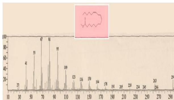
Fig. 2: Mass spectrum of 9,12-octadecadienoic acid methyl ester.
