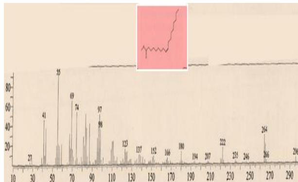
Fig. 3: Mass spectrum of 9-octadecenoic acid methyl ester.
