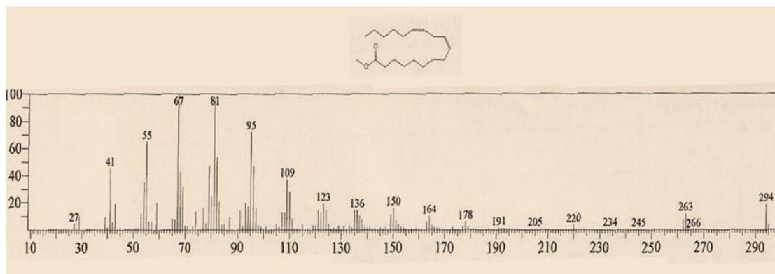
**Fig. 2: Mass spectrum of 9, 12-octadecadienoic acid methyl ester.**
