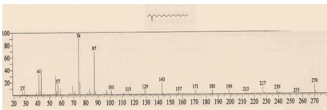
**Fig. 3: Mass spectrum of hexadecanoic acid methyl ester.**
