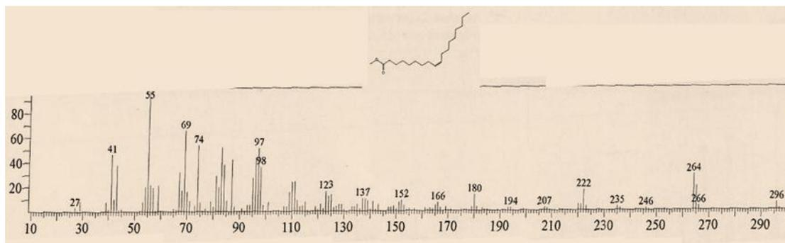
**Fig. 4: Mass spectrum of 9-octadecenoic acid methyl ester.**
