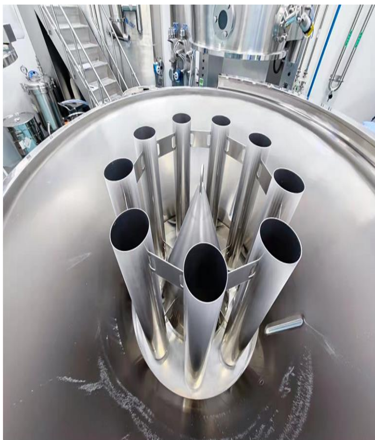
Figure 6: Fluid Bed Processor and Partition Columns.
