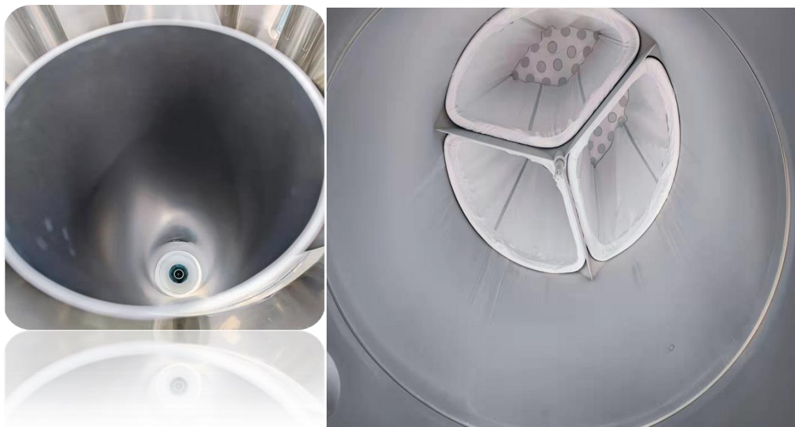
Figure 7: Nozzle Gun and Filer Bag
