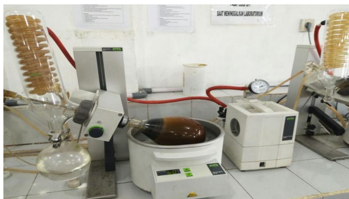
Figure 1: The process of making jubirkurihlah extract using the "Rotary Evaporator"
