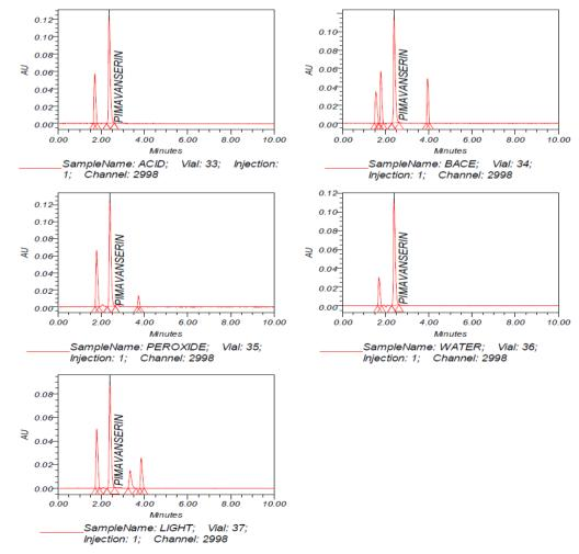
Figure 8: Forced degradation study of Pimavanserin.
