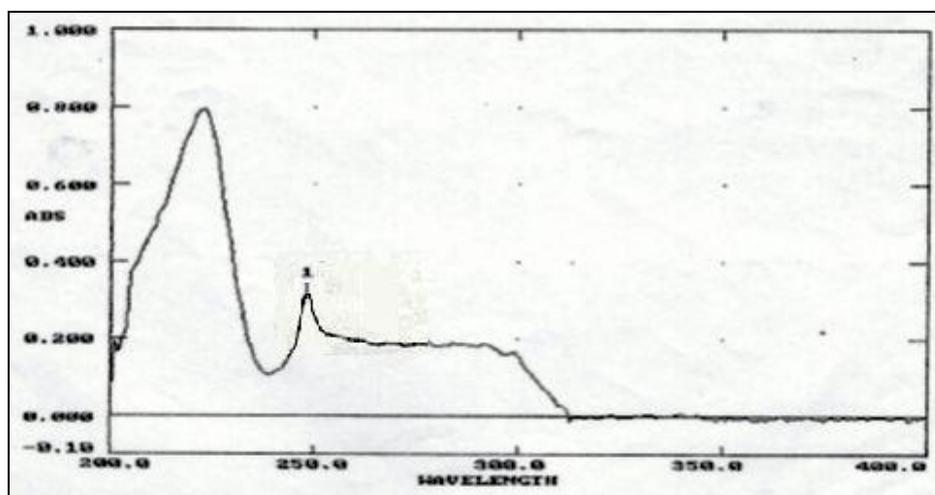
Fig.2: UV Visible Spectrum of Bilastine at 248nm.
