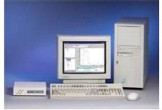
This is a computer that helps control all the modules of the HPLC instrument, takes the signal from the detector and uses it to determine the time of elution (retention time) of the sample components (qualitative analysis) and the amount of sample (quantitative analysis.
