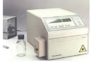
This is used for detecting individual molecules that comes out from the column. There are different varieties of detector that are used for deciding when the chemical should exit from the column.
