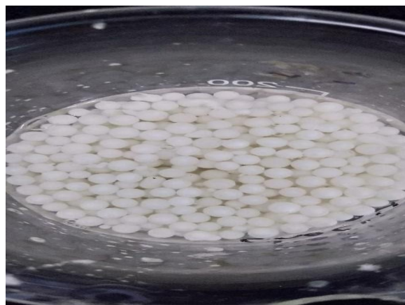
Figure 1: Shows immobilization of Xylanase in PVA-alginate matrix.
