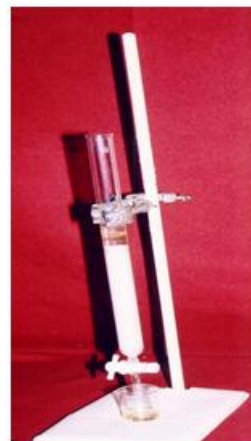
Fig. 4: Running condition in silica gel column chromatography.
