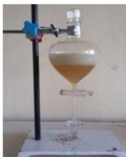
Fig. 2: Extraction of antimicrobial compound with ethyl acetate from the fermented broth.
