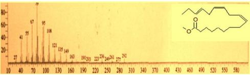
Fig. 6: The mass spectrum of 9,12,15-octadecatrienoic acid methyl ester.
