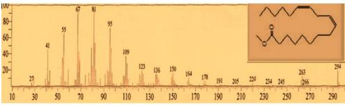
Fig. 5: The mass spectrum of 9,12-octadecadienoic acid methyl ester.
