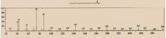
Fig. 7: Mass spectrum of methyl stearate.
