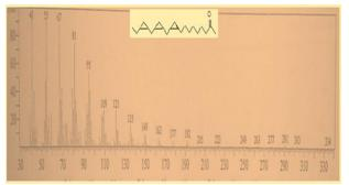
Fig. 5: Mass spectrum of cyclpropaneoctanoic acid methyl ester.
