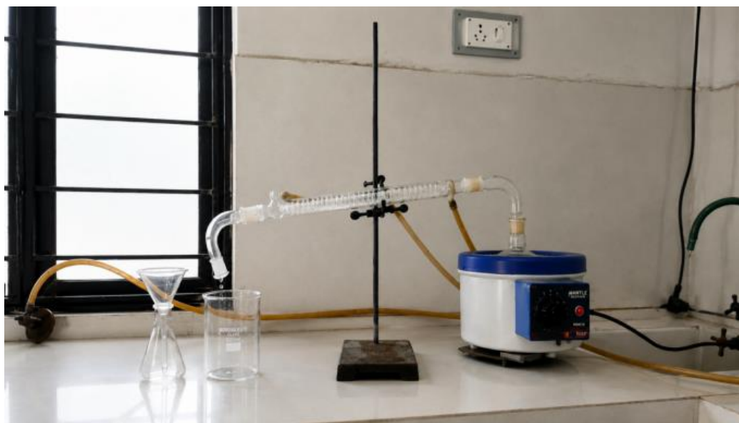
Figure 3: Hydro-distillation process of extraction of vetiver hydrosol from vetiver roots.
