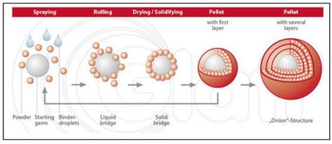
Figure 4 : Solution Layering.
