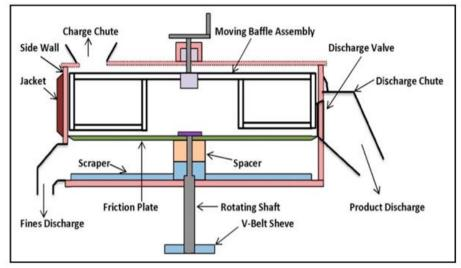
Figure 7: The spheronizer.
