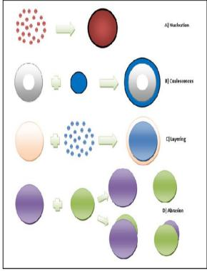
Figure 2: Pellet Growth Mechanism.
