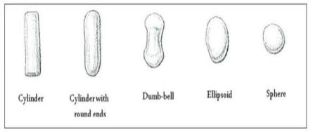
Figure 6: Schematic Representation Of Different Pellet Formation Stages During.
