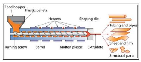
**Figure 5: Extrusion Process.**
