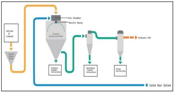
Figure 9: Spray Drying and Spray Congealing.
