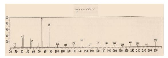
Fig. 3: Mass spectrum of hexadecanoic acid methyl ester.
